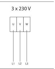
The inline fan is equipped with a variable speed motor. CFIR200 requires 3 x 230 V AC.
