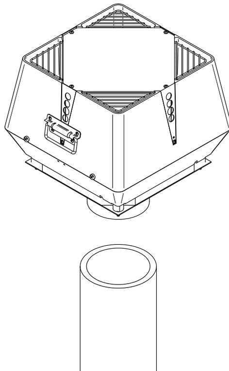
Use the safety wire to secure the fan to the chimney. Apply the supplied self-cutting screw in steel chimney. Then mount the wire through the designated hole in the base plate and into the wire lock.
